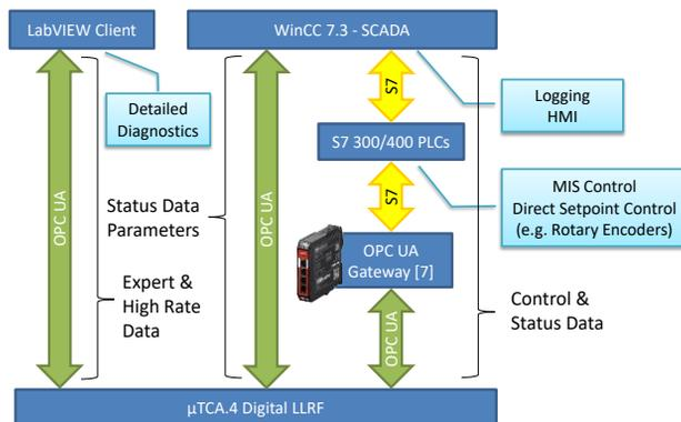
Figure 2: Digital LLRF communication scheme at ELBE
