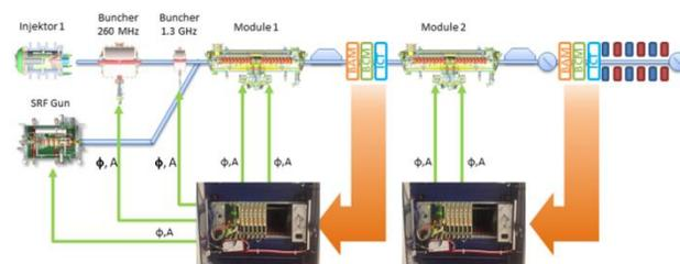
Figure 4: Feedback scheme for ELBE.
