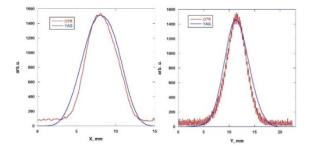
Figure 5: Horizontal and vertical beam profiles obtained from OTR and YAG images. Beam energy is 300 keV.
