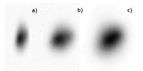
Figure 4: Raw OTR image (a), OTR image transformed to the beam coordinate space (b), YAG image (c). Beam energy is 300 keV.
