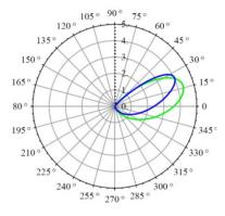
Figure 1: OTR intensity emitted at 90° to the beam direction as function of the angle  $\boldsymbol{\psi}$  for beam energies 100 keV (green) and 300 keV (blue). Data plotted by the green line were multiplied by a factor of 3.
