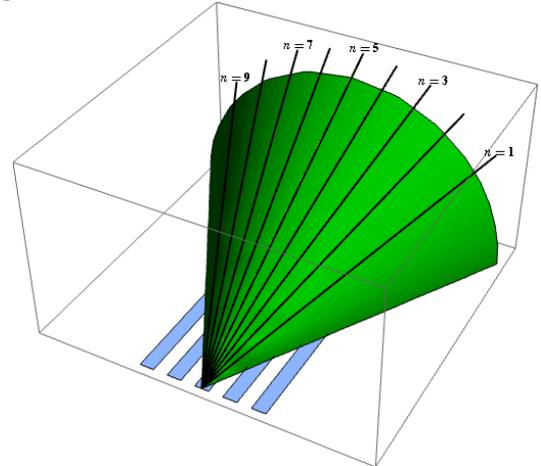
Figure 3: Conical distribution of Smith-Purcell radiation. The black lines correspond to the Smith-Purcell peaks.
