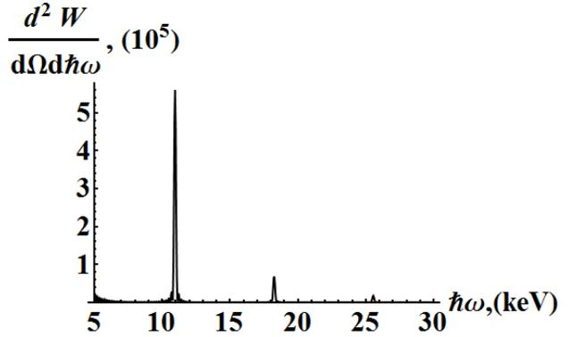
Figure 5: The distribution of X-Ray SPR over the conical surface at  $\theta = \arccos(\beta^{-1} \sin \alpha)$ ,  $\phi = 5^\circ$ . Here  $\gamma = 2 \cdot 10^6$  (electron energy  $E = 1\text{TeV}$ ),  $\hbar\omega_p = 26.1\text{eV}$  (beryllium),  $d = 0.1 \mu\text{m}$ ,  $a = 0.05 \mu\text{m}$ ,  $h = 1 \mu\text{m}$ ,  $\alpha = 30^\circ$ ,  $N = 20$ ,  $N_e = 10^{10}$ ,  $r_0 = 1 \mu\text{m}$ ,  $l = 60 \mu\text{m}$ .
