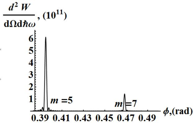
Figure 4: The distribution of X-Ray SPR over the conical surface at  $\theta = \arccos(\beta^{-1} \sin \alpha)$ . Here  $\gamma = 2 \cdot 10^6$  (electron energy  $E = 1\text{TeV}$ ),  $\hbar\omega_p = 26.1\text{eV}$  (beryllium),
