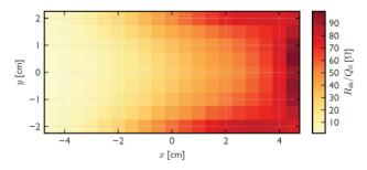
Figure 2: Measured shunt impedance of the rectangular Schottky monitor prototype.
