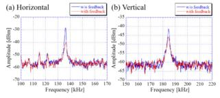
Figure 6: Tune spectra for the (a) horizontal and (b) vertical directions excited by the tune measurement system. The origins of a few peaks on the lower-frequency side of the horizontal tune are unknown.
