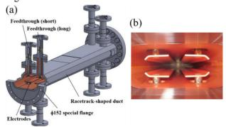
Figure 4: (a) Schematic drawing of the new stripline kicker duct and (b) photo of the inner electrodes.
