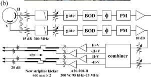
Figure 5: (a) Photo of the installed kicker ducts and (b) block diagram of the PF-AR feedback damper system. PM in the block diagram stands for pulse modulator.
