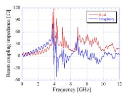
Figure 3: Real and imaginary parts of the longitudinal beam coupling impedance for the improved kicker. The simulated beam bunch length is 8.3 mm (28 ps).
