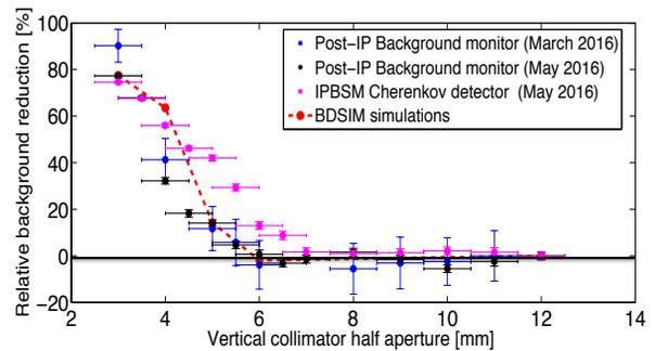
Figure 5: Comparison of the measured relative background reduction in the Post-IP region with the BDSIM simulations.
