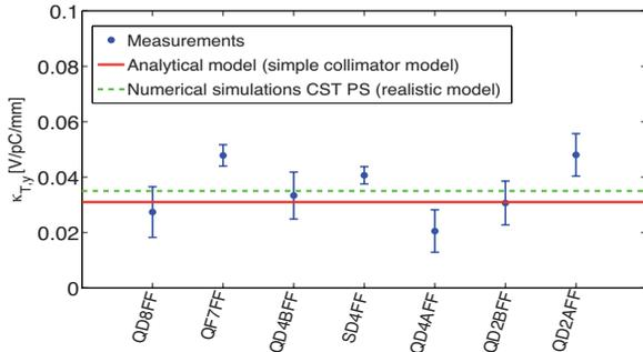
Figure 7:  $\kappa_{T,y}$  reconstructed at different C-BPMs from the 27th of May run.
