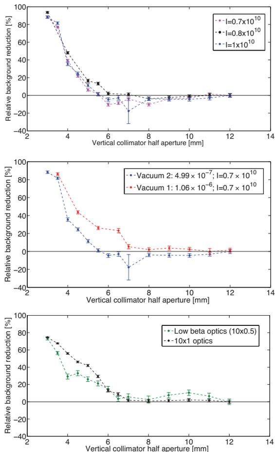
Figure 4: Relative efficiency for different intensities (top), DR vacuum pressures (middle) and optics (bottom).
