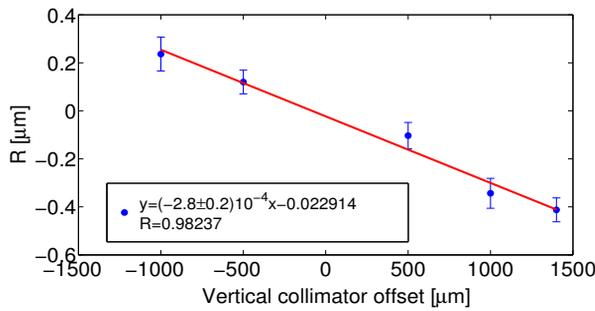
Figure 6: Residuals as a function of collimator offset from the 27th of May run at QF7FF.
