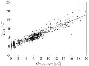
Figure 5: For the gas-jet based LPA, charge measured by the ICT versus charge measured by the Turbo-ICT. The line is a linear fit to the data.
