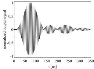
Figure 6: Normalized Turbo-ICT output signal measured on an oscilloscope.
