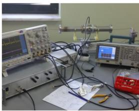
Figure 9: The BPM test setup.
