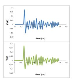
Figure 4: BPM output voltages from second (up) and fourth (down) antennas in time domain.
