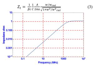
Figure 6: Antenna impedance distribution versus of the frequency.
