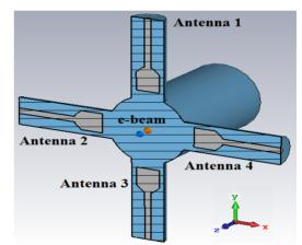
Figure 2: A view of button type BPM by CST.
