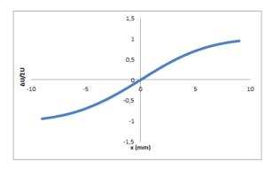
Figure 7: The resolution curve of designed BPM.
