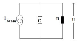
Figure 5: Equivalent circuit of BPM.
