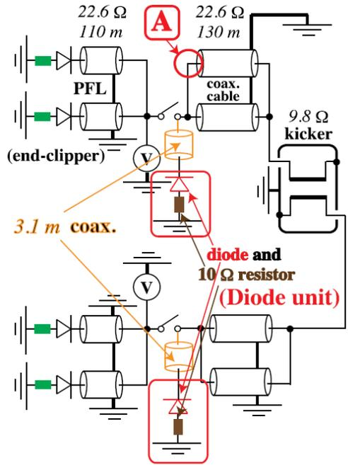
*3.1-m coaxial cables (connected to thyratrons)*
