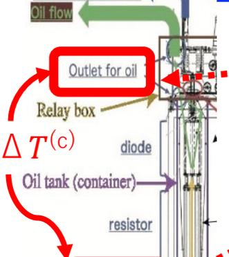
$$\Delta T^{(c)} = \frac{1000W[kW]}{r[\frac{g}{cm^3}] \frac{1}{60} V[\frac{L}{min}] 4.184 \bar{c}_p[\frac{cal}{gK}]}$$
