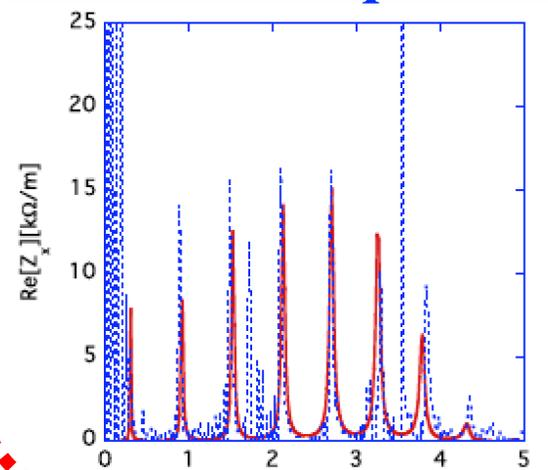
● However, it is the short plates in combination with the 130 m coaxial cables that create the resonance structure in the kicker impedance.
