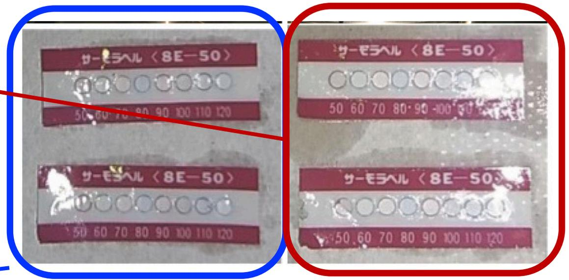
❖ No attached parts were heated beyond 50° C, which aligns with simulations.
