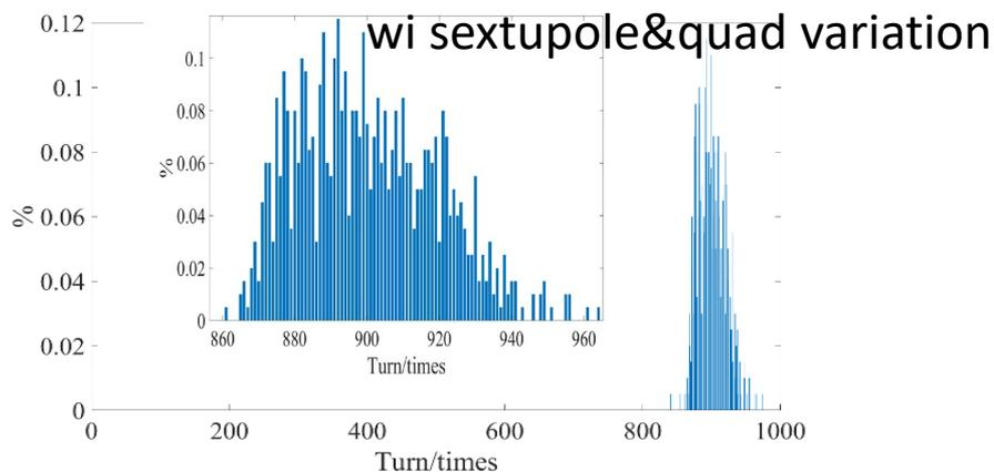
By tuning skew sextupole&Quad, the extraction rate can exceed 0.03% per turn
