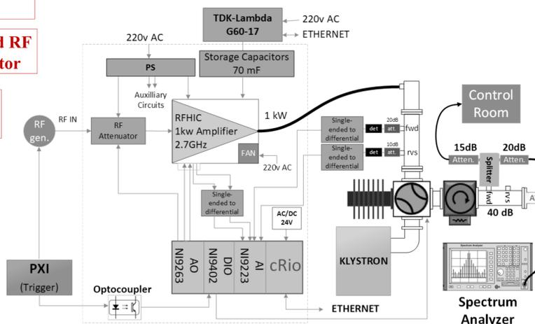
Injector SSPA-based amplification system scheme
