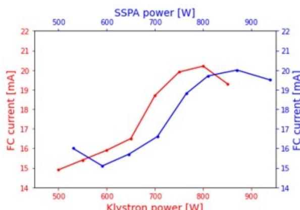
Beam extraction comparison between SSPA system and Klystron at different output power
