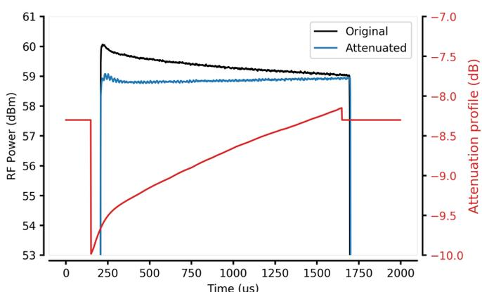
Variable attenuation control signal example
