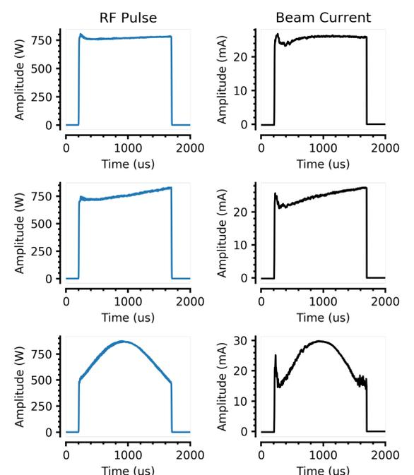
SSPA system beam extraction at different pulse shapes
