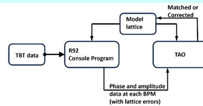
Figure 1: Flowchart from the TBT data to the interaction between R92 console program and the TAO.
