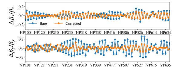
Figure 4: The difference between measured and design  $\beta$  functions before and after corrections
