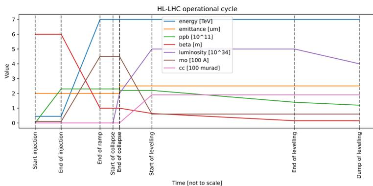
Figure 1: Schematic evolution of main quantities throughout the an HL-LHC cycle for proton
