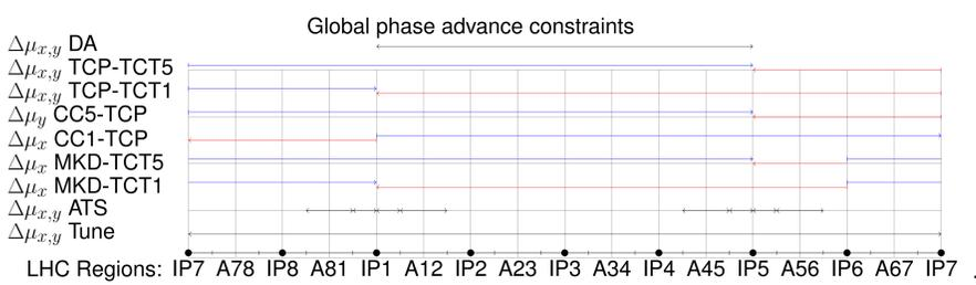
Figure 2: Phase-advance constraints considered during optics design during physics, for Beam 1 (blue), Beam 2 (red) and both beams (black). The LHC has the flexibility to change the phase advance in the 8 arcs and 16 half-straight sections around the IP. Although tune and ATS are strict constraints, the others could be fulfilled with some flexibility, which allows for some optimisation.
