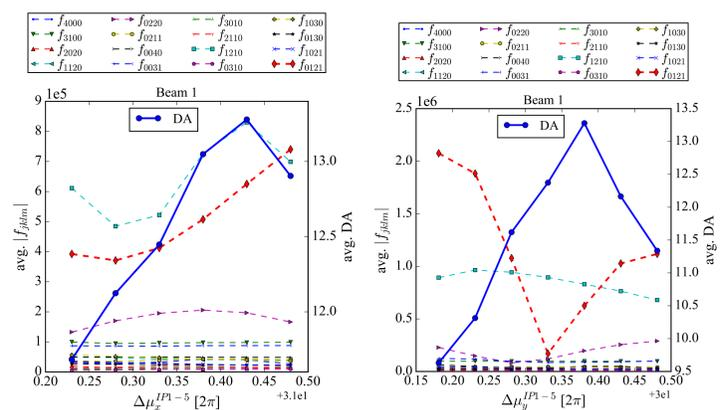
Figure 3: Octupolar resonance driving terms (RDT) and average dynamic aperture (DA) as a function of the horizontal (left) and vertical (right) phase advance between IP1 and IP5 (left) for the 15 cm  $\beta^*$  round baseline optics at the end of levelling. The DA is simulated without multipolar imperfections, with crossing angle, dispersion correction, and Landau octupoles set to their maximum strength of -570 A, after  $10^6$  turns and calculated over 60 angles.
