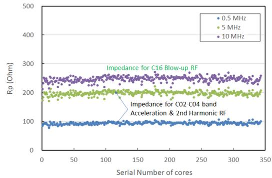
Figure 5: Impedance of all cores for PS booster.
