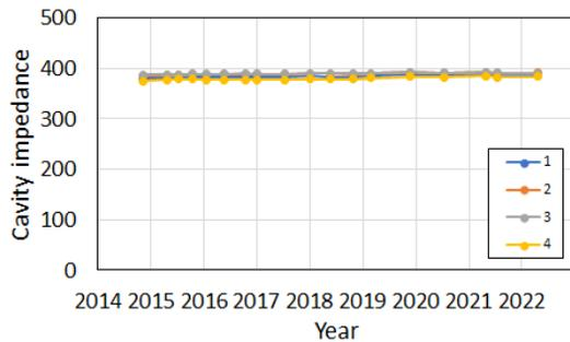
Figure 4: Impedance of MR cavities during 9 years. Four cavities using magnetic-annealed cores were installed in 2014. No significant variation was observed.
