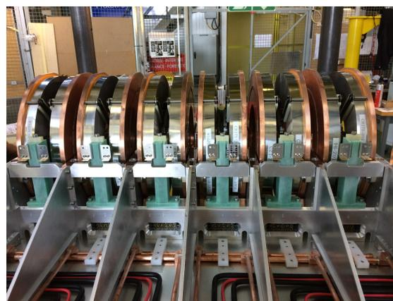
Figure 2: Indirect cooling cavity of PS booster. Cores are mounted on the copper cooling discs.
