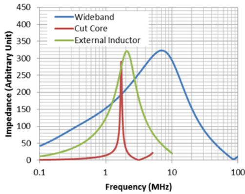
Figure 3: Bandwidths of the wideband cavities controlled by the cut-core scheme and external inductor.
