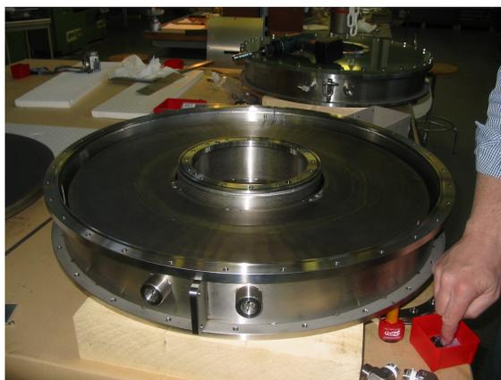
Figure 1: Water-proofed magnetic alloy cores in the water tank of LEIR cavity.
