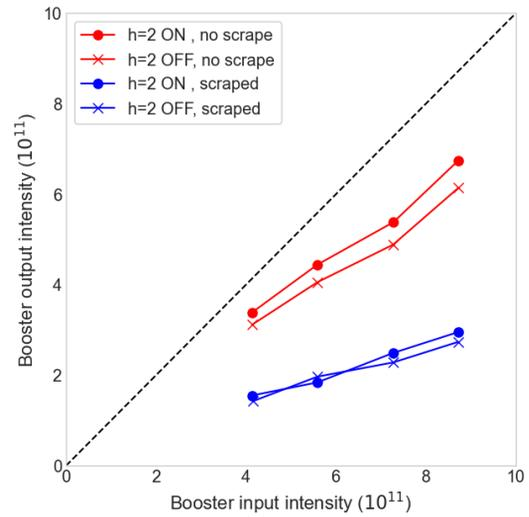
Figure 7: Booster transmission improvement with  $h=2$ . Dashed line indicated case of perfect transmission.
