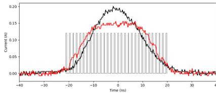
Figure 12: RHIC bunches at 3.85 GeV/n with only a 9 MHz voltage (black) and with 9 MHz plus 28 MHz defocusing voltage (red). The LEReC electron bunch structure (gray) shows the 30 bunches with 704 MHz spacing and 0.4 ns bunch widths.
