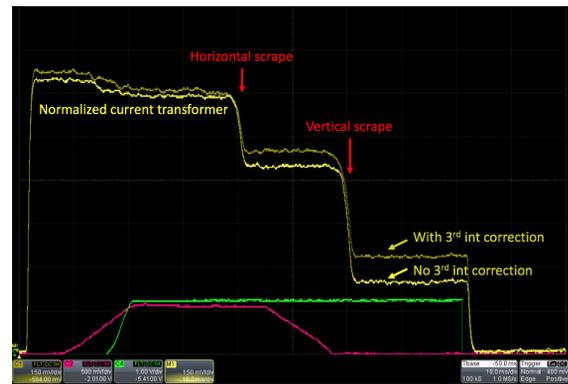
Figure 8: Booster intensity transmission through transverse emittance scraping with and without third integer stopband correction.
