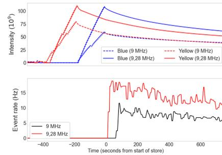
Figure 13: Intensity and luminosity comparison for two RHIC 3.85 GeV/n gold fills with and without bunch flattening using the 28 MHz RF. Intensity is shown for both the Blue and Yellow rings. Event rate is from the STAR detector. Extracted intensity from the AGS was the same in both cases.
