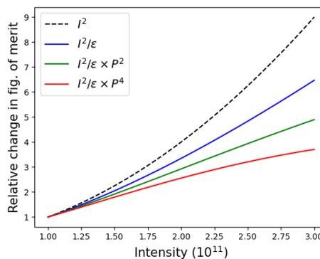
Figure 4: Predicted relative change in polarized collider figures of merit assuming the emittance and polarization are independent of intensity (black), the emittance dependence of Fig. 3(a) (blue) and both the emittance and polarization deterioration of Fig. 3(a,b), for transverse (green) and longitudinal (red) spin physics programs.
