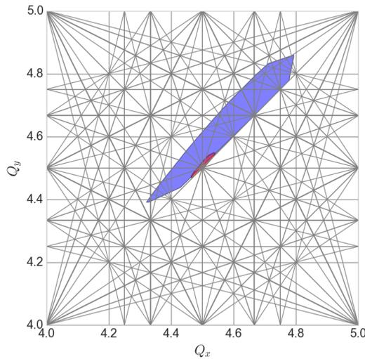
Figure 6: Booster tune footprint (with resonances up to 5<sup>th</sup> order) from direct space charge for coasting beam just after injection (red) and for bunched beam just after capture into  $h=1$  (blue).
