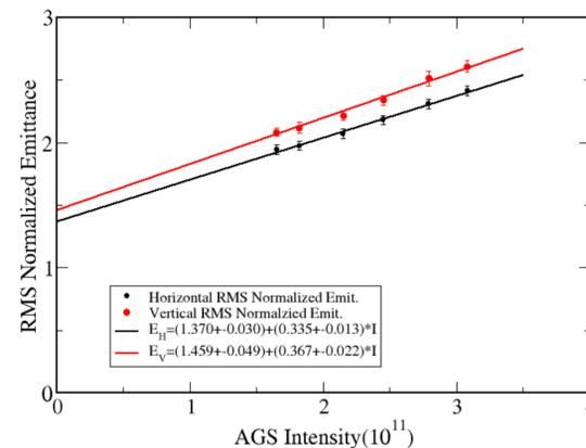
Figure 3: (a) Polarization and (b) transverse emittances as functions of AGS extraction intensity.
