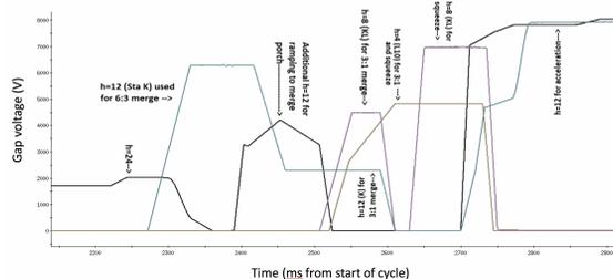
Figure 10: Voltage program for merges for to 6→3 and 3→1 merges for Au beam in the AGS. As shown there is an acceleration from injection energy ( $\gamma = 1.11$ ) to an intermediate porch ( $\gamma = 1.17$ ) between the first and second merges (2400–2500 ms). The increased energy alleviates the peak space charge forces after the second merge.
