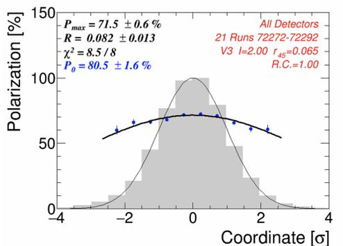
Figure 2: Horizontal polarization profile measured with a thin carbon target at AGS extraction. Intensity profile is shown in gray. The polarization (blue) decreases toward the edges of the intensity profile due to intrinsic depolarizing resonances.
