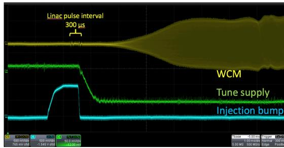
Figure 5: The Booster injection process. As soon as the 300  $\mu$ s Linac pulse ends, the circulating beam is steered off the injection foil to prevent more scattering. The tunes are raised away from the half-integer before the beam is bunched.
