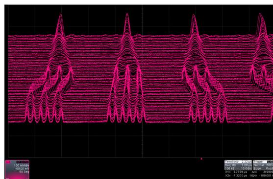
Figure 11: Wall current monitor measurement during the AGS 6→3→1 merges. (Each trace shows more than one turn).
