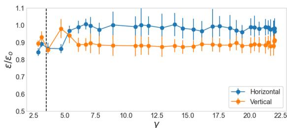
Figure 9: Relative change in transverse emittances in AGS when the peak current is reduced from injection ( $\gamma = 2.5$ ) through  $\gamma = 3.5$  (marked with vertical dashed line).
