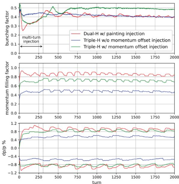
Figure 3: The longitudinal beam simulation results for the dual-harmonic and triple-harmonic operations [15]. The top, middle, and bottom figures show the BF, momentum filling factor, and  $dp/p$ , respectively. The horizontal axis corresponds to the number of turns. The details of each parameter are explained in Ref [15].
