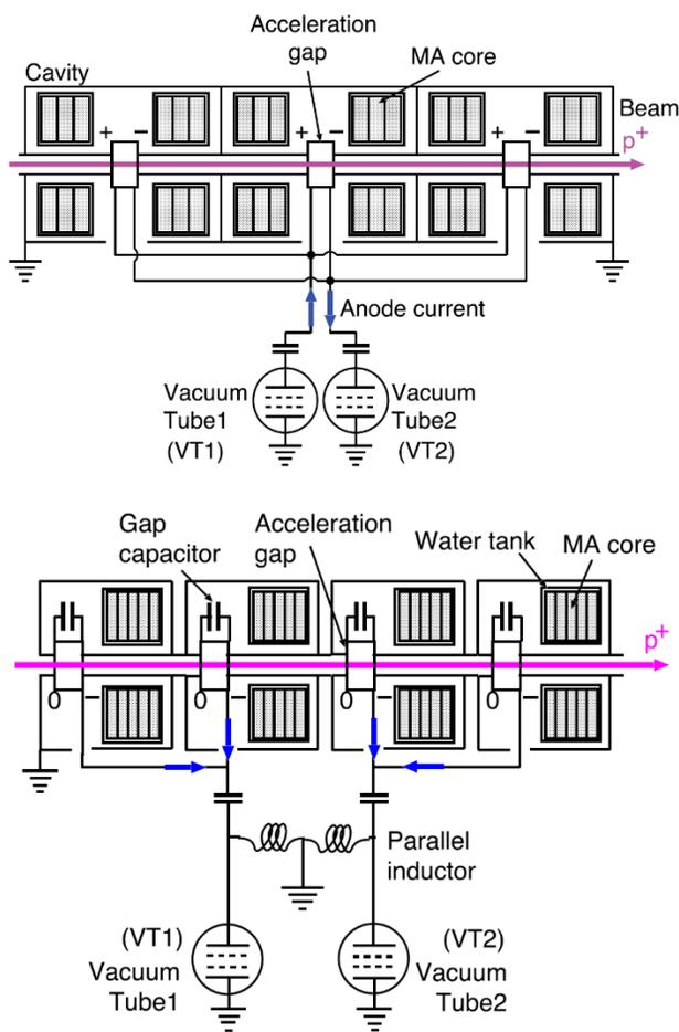
Figure 2: Schematic view of the RCS cavity [4]. Upper figure shows the conventional RCS cavity system in the push-pull operation. Lower figure shows the new single-ended RCS cavity.
