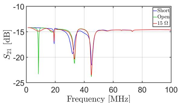
Figure 7: Magnitude of simulated  $S_{21}$  parameter versus frequency up to 100 MHz with different electrical cable terminations: short circuit in blue, ideal open transmission line in green and  $15\ \Omega$  resistor in red.
