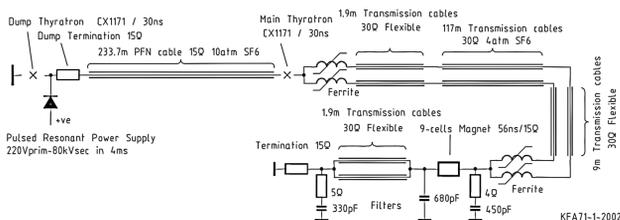
Figure 6: Circuit schematic of a magnet module unit. The output of each module, indicated as "9-cells magnet", is connected to a  $15\ \Omega$  resistive termination [16].
