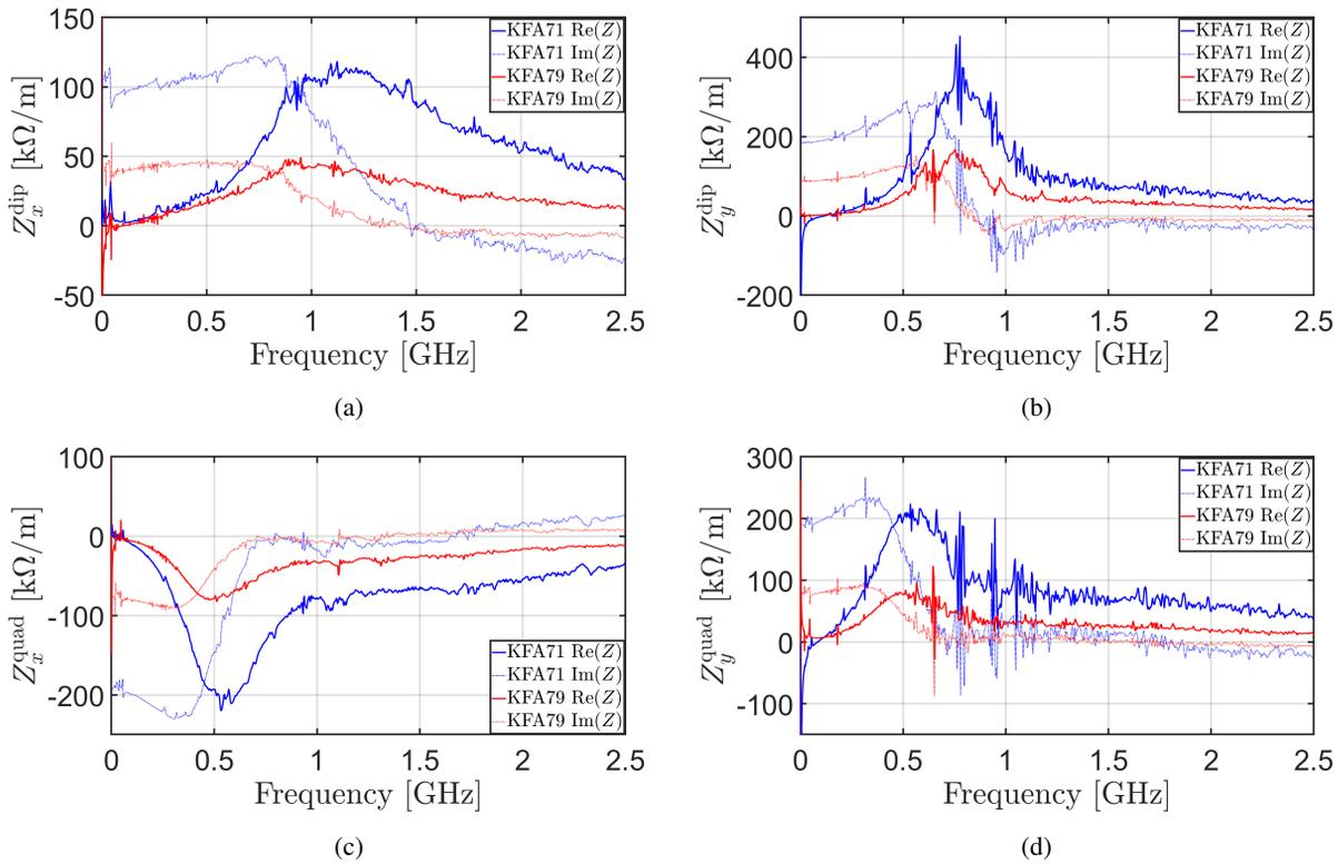
Figure 5: Real and imaginary part of the transverse dipolar horizontal (a) and vertical (b) and quadrupolar horizontal (c) and vertical (d) beam coupling impedance of KFA71 (blue) and KFA79 (red).
