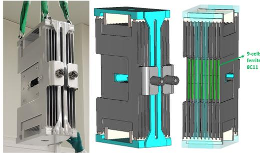
Figure 1: Photo (left) and 3D geometry (right) of a single module of the kicker magnet KFA79, with the assembly of aluminum alloy plates and nine cells of ferrite.
