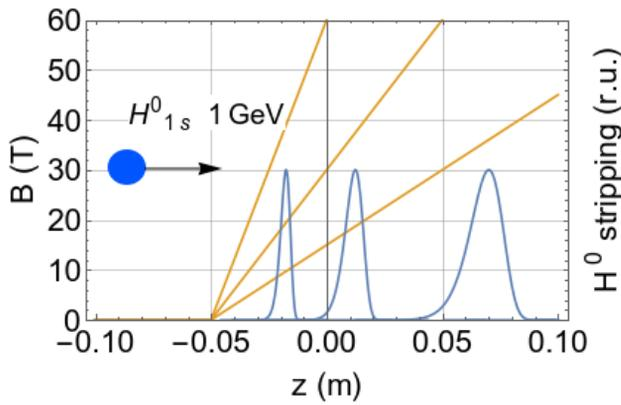
Figure 3: Stripping of  $H^0_{1s}$  neutral hydrogen beam with 1 GeV energy in a different transverse magnetic fields. Lower curves show stripping rate/probability distribution along  $z$ -direction of the  $H^0$  atom.
