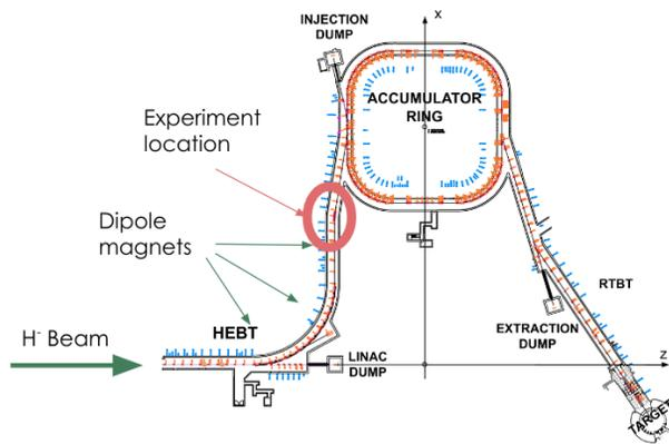
Figure 6: Schematics of SNS injection system, location of the LACE experiment and beam transportation.
