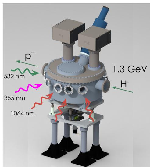
Figure 9: Design of experimental vessel for the next series of LACE experiments in LINAC area for 1.3 GeV  $H^-$  beam.
