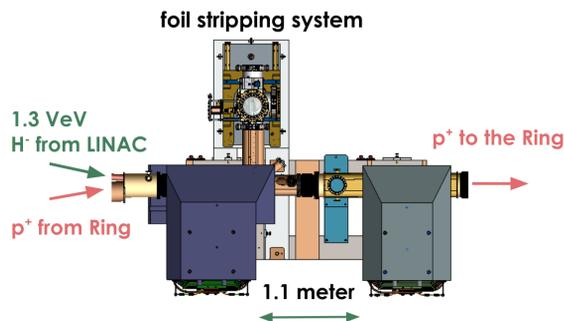
Figure 8: Foil operated design of the injection area for 1.3 GeV proton power upgrade PPU project [12].
