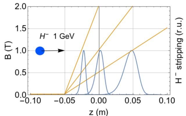
Figure 2: Stripping of  $H^-$  beam with 1 GeV energy in a different transverse magnetic fields that linearly grow from left to right. Lower curves show stripping rate/probability distribution along  $z$ -direction of the  $H^-$  ion.
