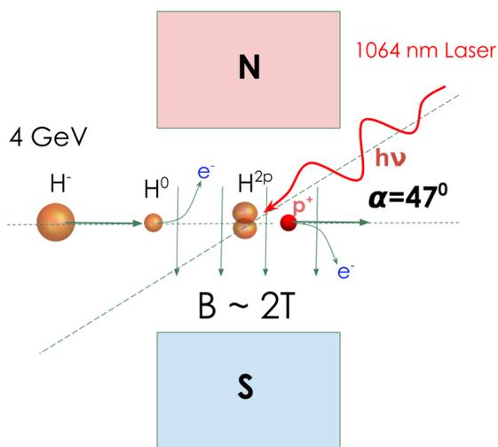
Figure 7: The most optimal LACE scheme for 4GeV beam.
