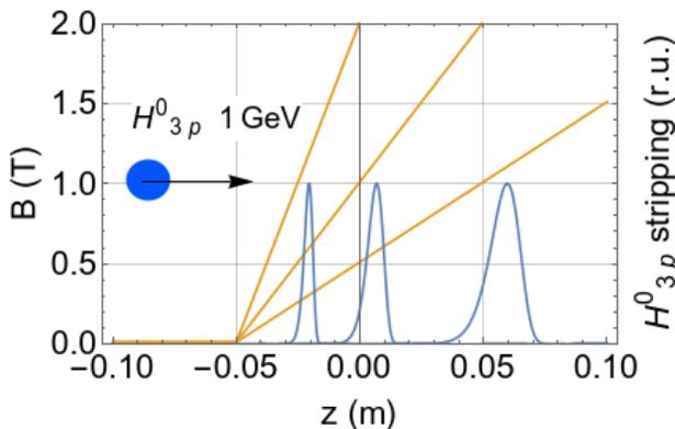
Figure 4: Stripping of  $H^0_{3p}$  neutral hydrogen beam with 1 GeV energy in a different transverse magnetic fields. Lower curves show stripping rate/probability distribution along  $z$ -direction of the  $H^0$  atom.
