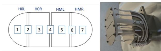
Figure 4: The  $H^0H^-$  monitor consists of four plates and is installed in front of the dump. The plates signal calibration is performed using a BCT at the end of the TL and moving the injected beam on the seven sketched positions.
