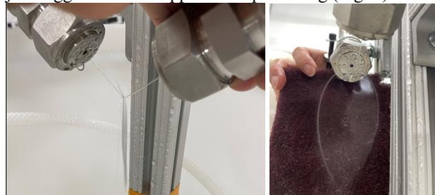
Figure 2: Water film produced by colliding two jets from 1-mm diameter nozzles.
