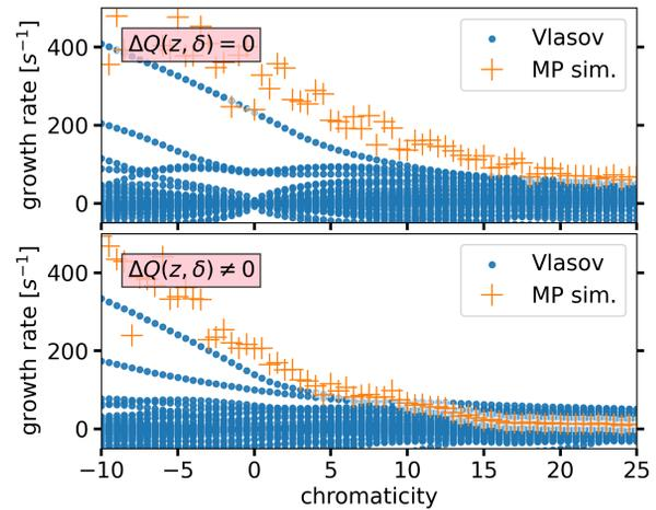
Figure 4: Instability growth rate from macro particle simulations (orange) and from calculated Vlasov modes (blue) as a function of chromaticity for only dipolar force (top) and with detuning from e-cloud (bottom).
