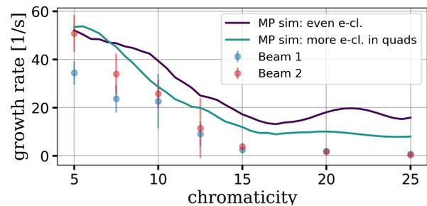
Figure 5: The instability growth rates from measurement of beam 1 (blue) and beam 2 (red) for several values of chromaticity. The simulated growth rates assuming even e-cloud formation in dipole and quadrupole magnets (indigo) and assuming slightly more e-cloud in quadrupoles (teal).
