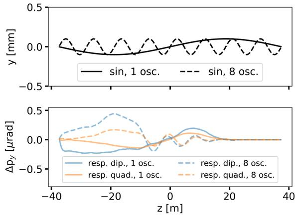
Figure 2: Two sinusoid bunch distortions (top) of varying number of oscillations along the bunch and the corresponding response functions (bottom) generated by e-cloud in dipoles, blue, and in quadrupoles, orange.
