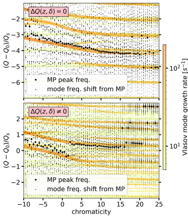
Figure 3: The mode frequency shift vs. chromaticity for simulations with (bottom) and without (top) the detuning term,  $\Delta Q(r, \phi)$ , from e-cloud. The calculated Vlasov modes are plotted as green-yellow-orange and the spectra from the macroparticle tracking is plotted as black dots.
