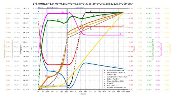
Figure 2: Main parameters of the RFQ.
