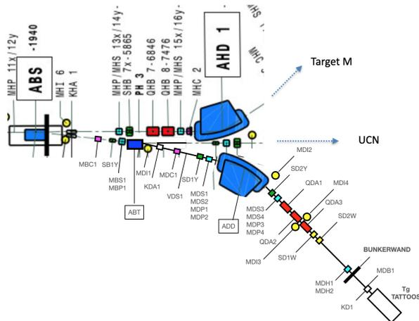
Figure 2: Main components along the proposed TATTOOS beamline. Beam loss ionisation chambers are depicted with yellow circles; bending magnets in blue; steerer corrector magnets in green; quadrupole magnets in red; beam position and profile monitors in cyan; beam current monitors in pink; wobbler magnets in yellow; collimator MDB1 in white.
