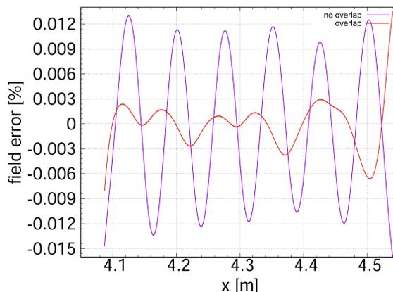
Figure 3: Field error along the radius line in the 2D model after current optimisation for no overlapped (purple) and overlapped trim coils (red).
