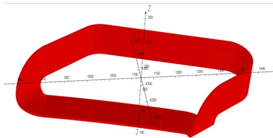
Figure 6: 3D model of one trim coil in OPERA software.
