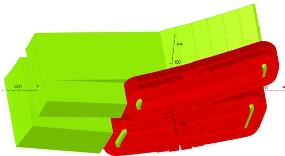
Figure 5: 3D model of the doublet in OPERA software.
