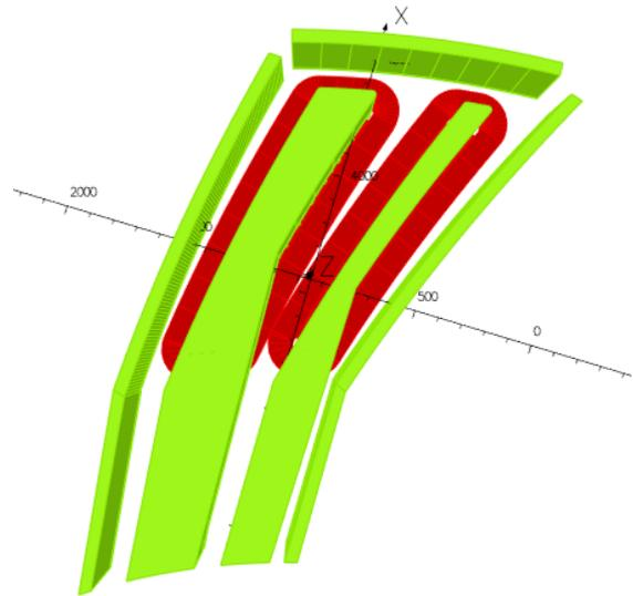
Figure 7: 3D model of the doublet in OPERA software with field clamps.
