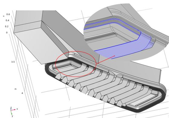
Figure 4: 3D model of overlapped trim coils for a single magnet in COMSOL software.
