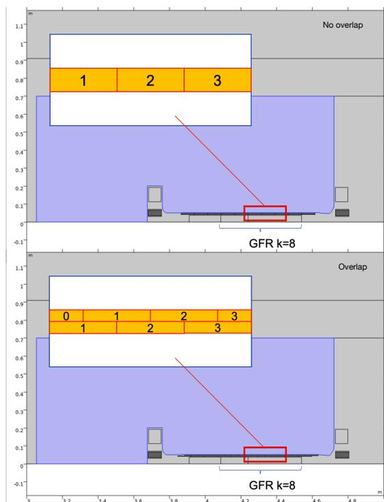
Figure 2: 2D model in COMSOL of no overlapped (top) and overlapped (bottom) trim coils.
