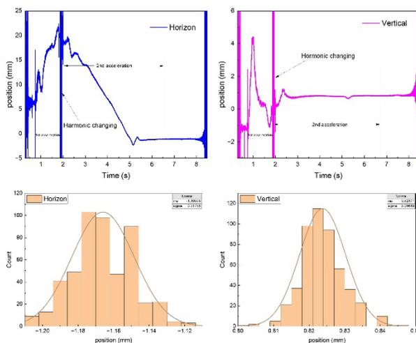
Figure 7: The beam position measured at CSRm and the root mean square. The left is the horizon position and the right is vertical.
