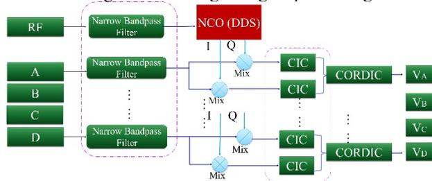
Figure 3: Digital signal processing.
