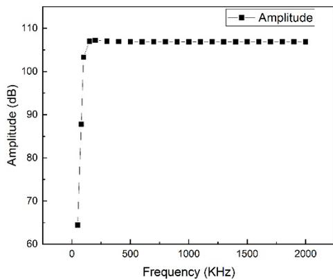
Figure 4: High-pass IIR filter amplitude-frequency response implemented by FPGA.
