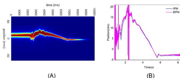
Figure 8: Compare with IPM in horizon position. (A) is the profile distribution horizon position of the beam, (B) is the beam position retrieved from IPM, and the BPM is detected.
