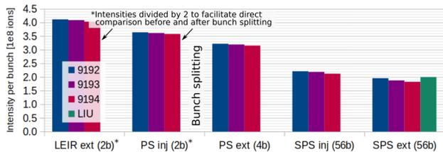
Figure 5: Bunch intensities across the ion complex for the first three LHC fills in 2023 together with the LIU target parameters [10] at SPS extraction.
