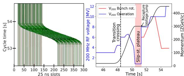
Figure 3: Left: Time (vertical axis) evolution of the 56 SPS bunches versus 25 ns slots on the slip stacking intermediate-energy plateau in SPS. Right: RF voltage functions (red, blue) are overlaid on top of main bending magnets’ field function (black). Red voltage function refers to the bunch rotation option, the blue voltage (w/o bunch rotation) is the operational baseline.
