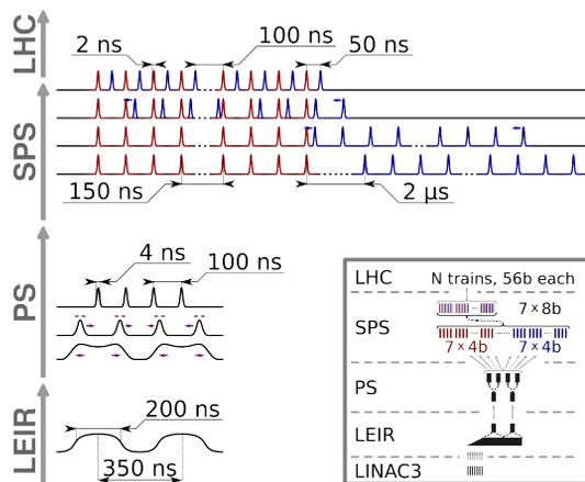
Figure 2: Evolution of longitudinal beam structure along the ion injector chain. The bunch spacings and lengths are indicative.
