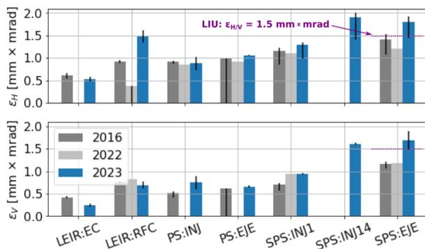
Figure 6: Evolution of horizontal and vertical normalized emittance between LEIR electron cooler (EC) and SPS ejection along with the LIU target [10]. The origin of reference data from 2016 is [2], and from 2022 is [1].
