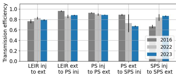
Figure 4: Transmission efficiencies in 2016, 2022, and beginning of the ion run in 2023.
