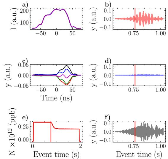
Figure 5: Transverse distribution (a) and vertical motion of the bunch when the instability was present (c). In (e), the plot shows the beam intensity, and the vertical line represents when the snapshot was taken in the event timeline. In (b), (d), and (f) the average motion of the beam was sampled at the center, head, and tail of the bunch, respectively.
