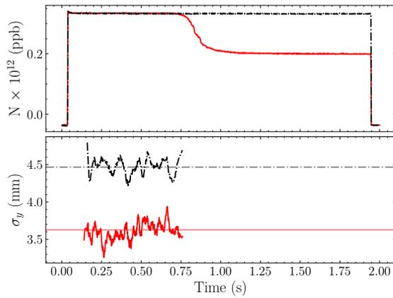
Figure 4: Beam intensity (a) and IPM data (b) when the beam size increased (dotted black) and without the beam size blowup (solid red).
