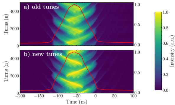
Figure 3: longitudinal profile of the beam over 5000 turns before the tune change (a) and after the tune change (b). The red trace in both (a) and (b) shows the average longitudinal profile over the same number of turns.
