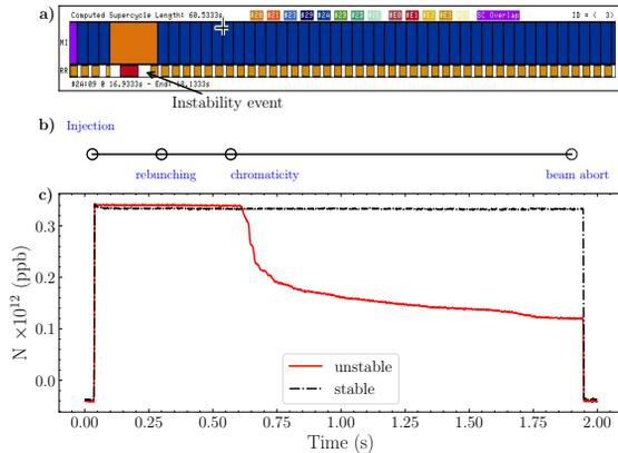
Figure 1: Operational supercycle with the instability event shown (a), the processes that occur during our study event (b) and beam intensity ( $N$ ) during two separate events (c). In (c) the red solid trace represents the intensity when the instability occurred, while the red dashed trace shows the beam intensity after the instability was mitigated by the tune change.
