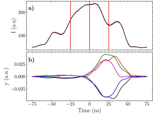
Figure 2: Transverse distribution along the bunch (a) and the beam vertical displacement (b) for 5 consecutive turns during an instability. The vertical lines in (a) represent  $\sim -\sigma_t$ , 0, and  $\sigma_t$  and are hereafter referred to as the head, center, and tail of the bunch, respectively.
