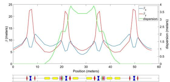
Figure 1: Twiss parameters of the RCS one super-period.
