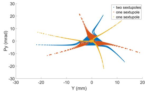
Figure 3: Resonance extraction due to skewsextupoles.
