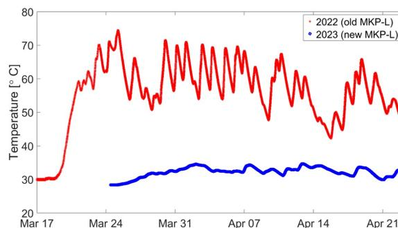
Figure 6: Comparison between the MKP-L heating over the 2022 and 2023 scrubbing runs in the SPS.
