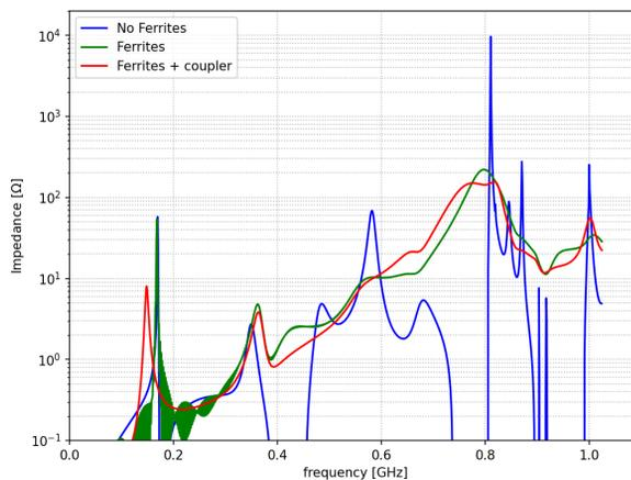
Figure 9: Longitudinal beam coupling impedance of the wire scanner without ferrites, with ferrites and with ferrites + coupler.
