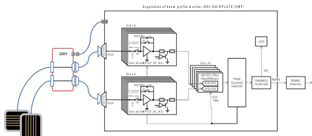
Figure 4: Structure from the SEM-grid wires to the FEE.
