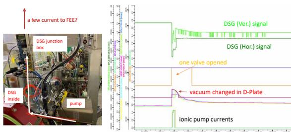
Figure 6: Possible spark event to destruct the DSG FEE.
