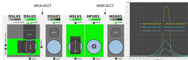
Figure 13: A typical scanning result with the slit and ACCTs (and/or HFU).
