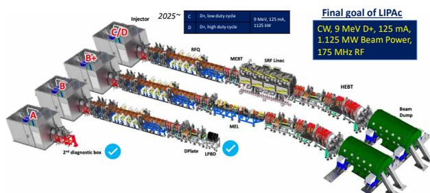
Figure 2: LIPAc beam operation phases.
