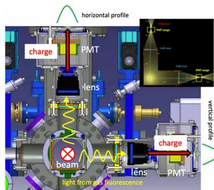
Figure 11: Schematic view of the inside of FPMs.
