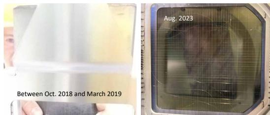
Figure 5: Broken wires during venting in the D-Plate.
