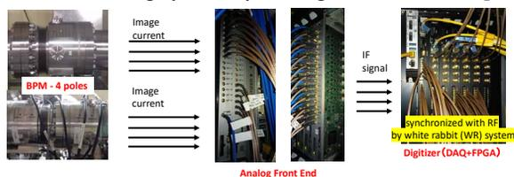
Figure 10: The BPM system and signal transfer structure.
