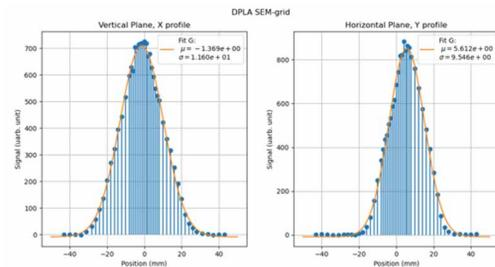
Figure 16: Full beam profile on the DSG.
