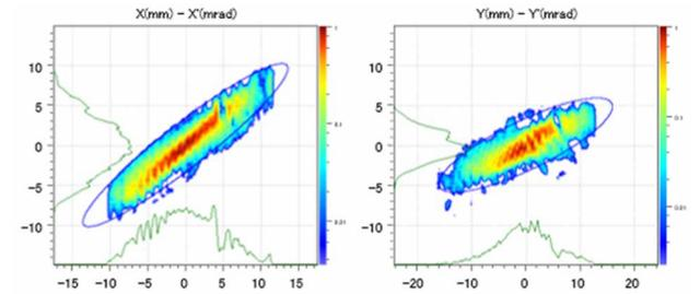
Figure 15: Result of the TraceWin simulation of the emittance using the parameter measured.
