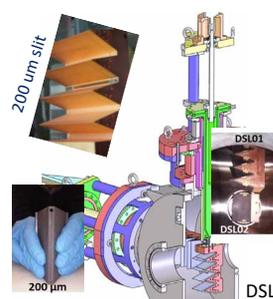
Figure 8: The structure of D-Plate slit (DSL).
