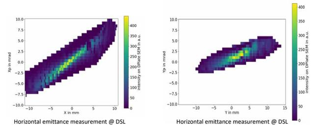
Figure 14: Emittance measurement with DSL and DSG during HEBT steering tuning.
