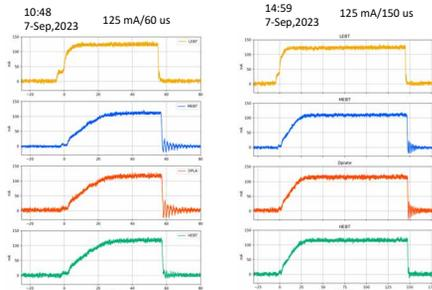
Figure 12: Beam transmission and waveform by ACCTs, from upstream (LEBT) to downstream (HEBT).
