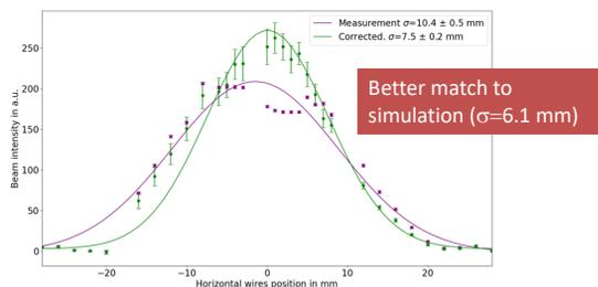
Figure 7: Example of beam profile before and after the gain correction.
