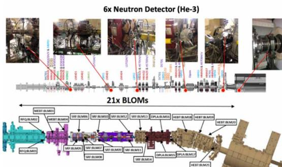
Figure 9: Positions of BLOMs and neutron detectors.
