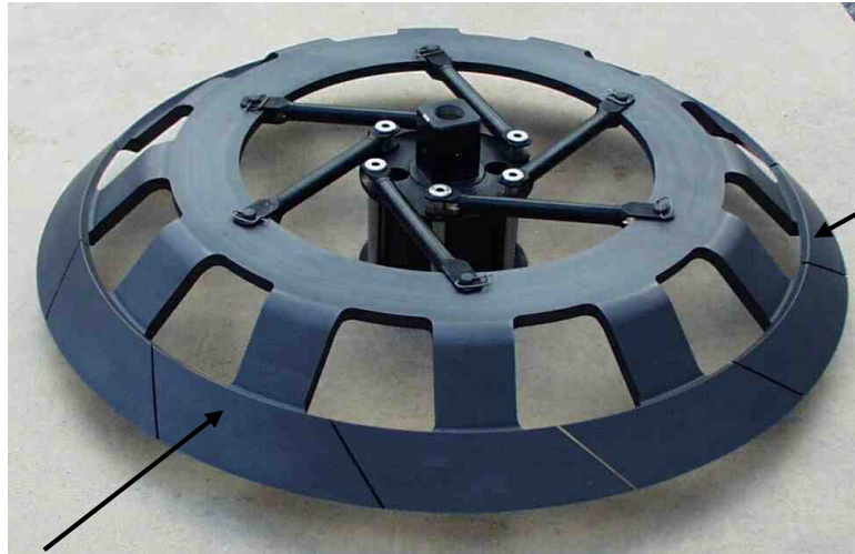
12 segments with 1 mm slit
