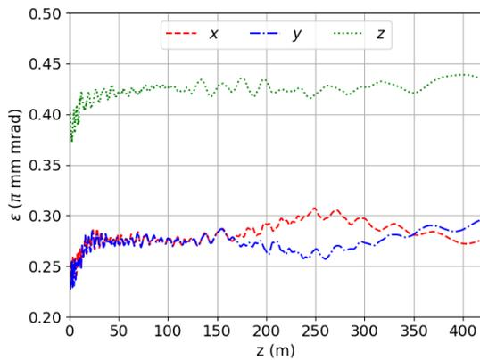
Figure 3: Normalized rms emittance in the linac.
