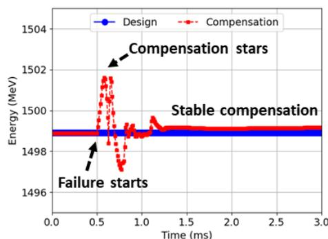
Figure 12: Final energy for the compensation case.
