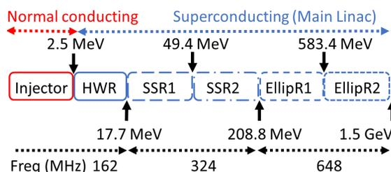
Figure 2: Linac lattice configuration.
