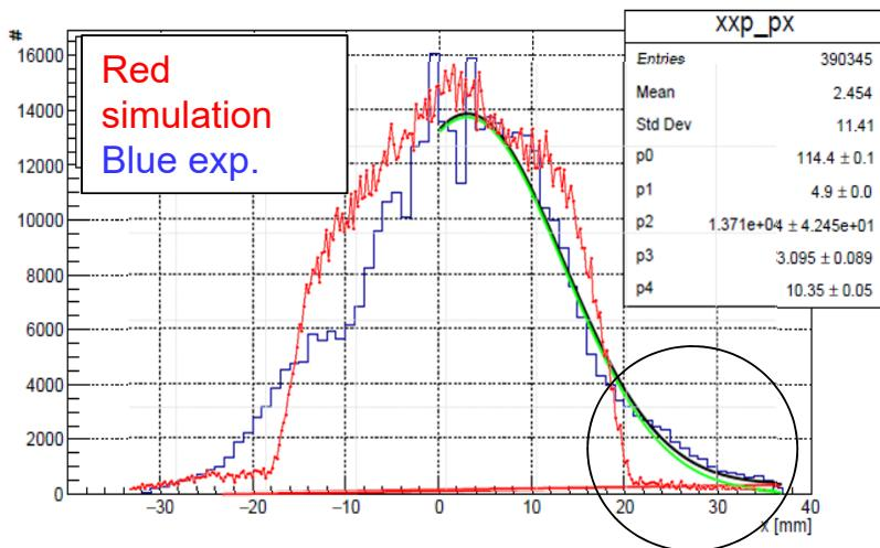
x-profile of 130 mA D beam at 100 keV
