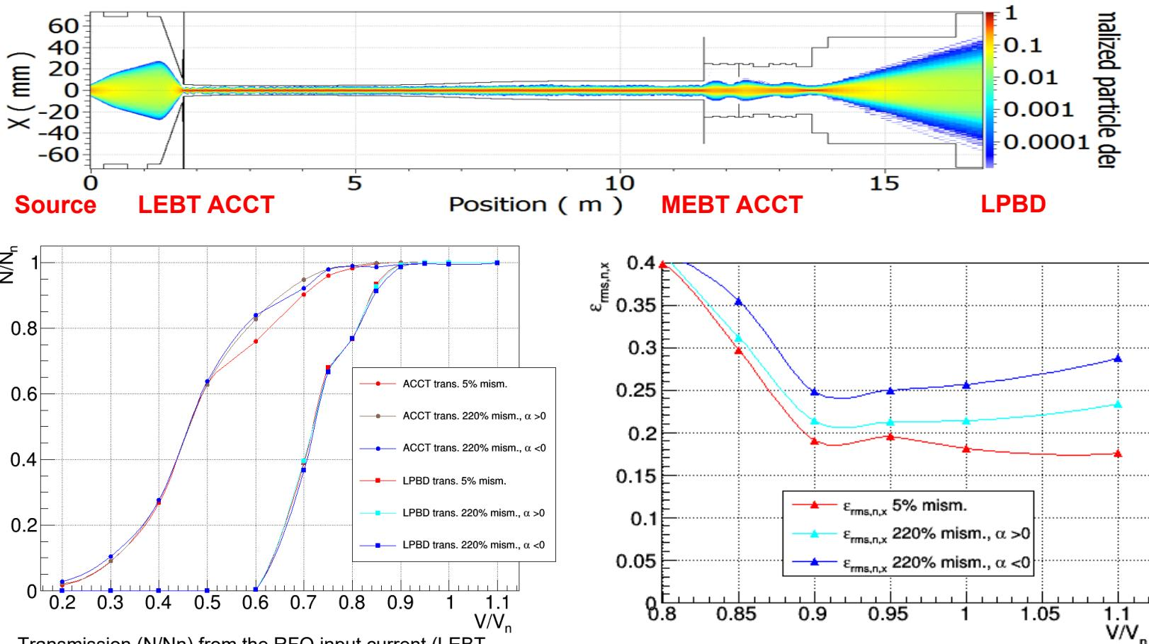
Transmission ( $N/N_n$ ) from the RFQ input current (LEBT ACCT) to the output of the RFQ (MEBT ACCT) and to the end of the line (LPBD) with respect to different RFQ voltage ratios normalized ( $V/V_n$ ).
