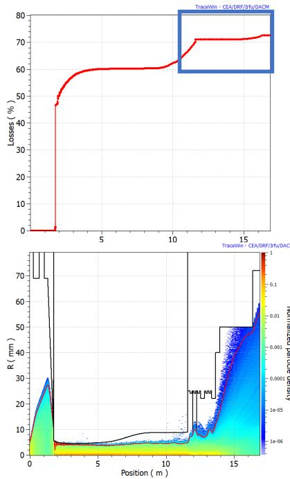
We loose half of the beam before the RFQ injection point. This may explain the half current at the ACCT respect to extraction.
