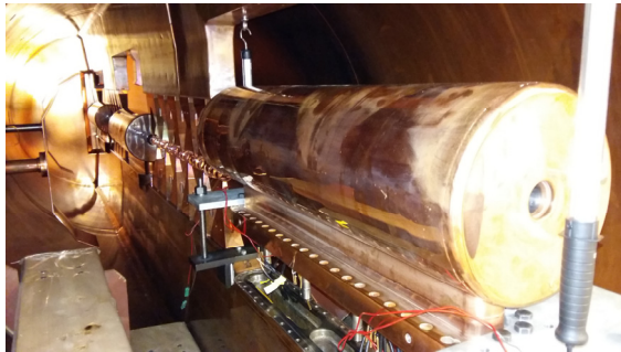
IH-cavities with KONUS (combined 0-degrees structure)
