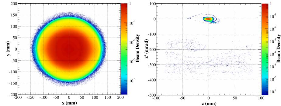
Phase spaces on the beam dump (1.1 MW)
