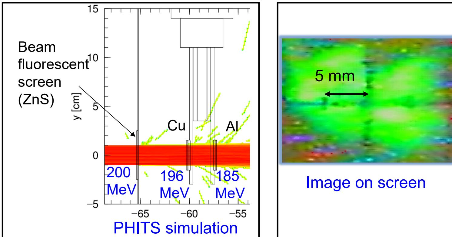
Adjusted beam area to cover sample with controlling magnetic field of magnets
