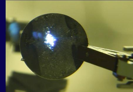
Pin holes at target of SNS (by B. Riemer)
