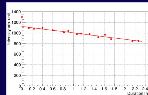
$\text{Al}_2\text{O}_3$  paint with low impurity: No degradation in short wavelength
