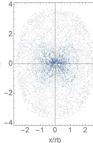
All points are plotted **in every S lattice period** (Poincare surface of section plots) with different particle initial conditions for propagation **over 300 lattice periods**
