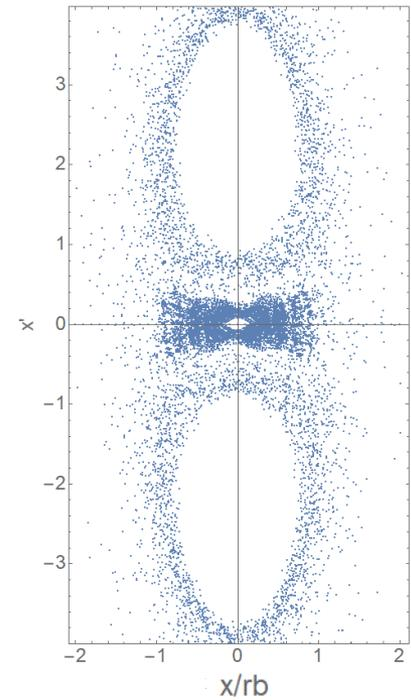
All points are plotted **in every S lattice period** (Poincare surface of section plots) with different particle initial conditions for propagation **over 300 lattice periods**
