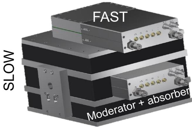
Assembly of a fast and a slow detector
