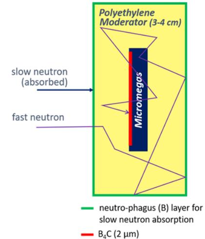
➔ “fast” detector (MM + H-rich target) appropriate for high flux - high energy neutrons
