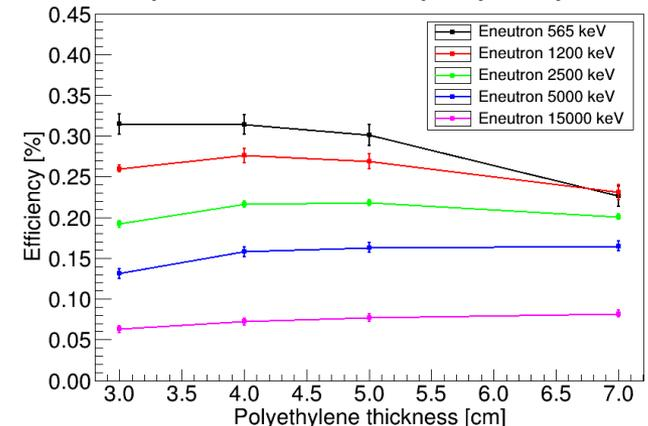
**Moderator thickness chosen for final detector: 5 cm**
