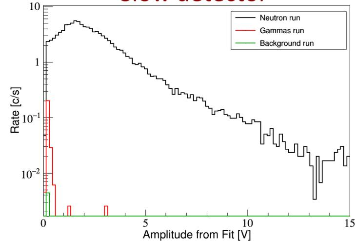
Applying an amplitude cut at 0.3 V →
