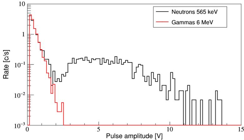
Applying an amplitude cut at 2 V →
