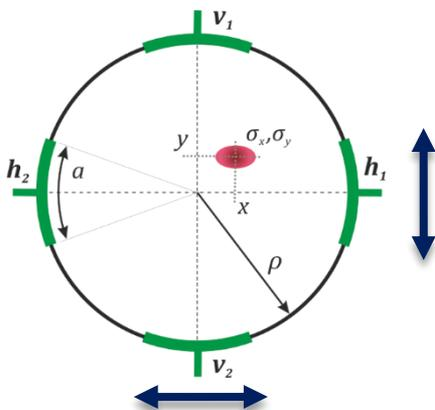
Measure beam position & align PU
