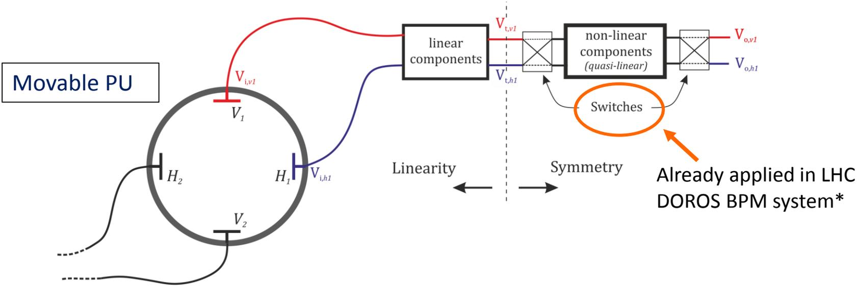
\*M. Gasior, "Calibration of a non-linear beam position monitor electronics (...)", Proceedings of IBIC 2013
