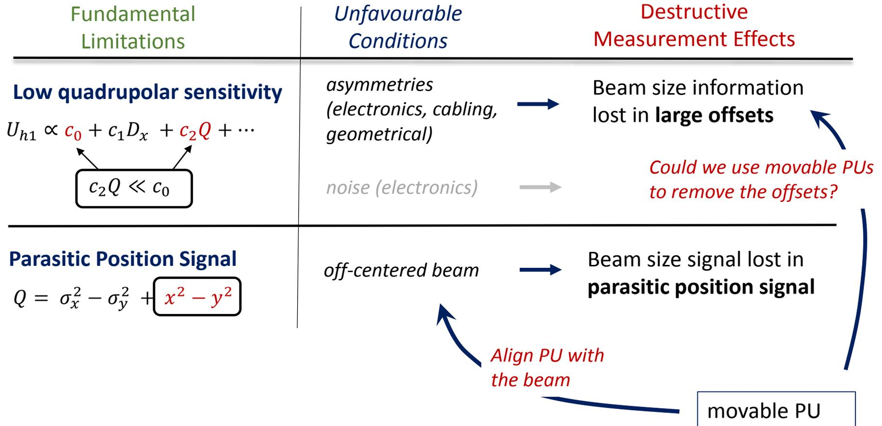
\*\* **Noise** from electronics may significantly affect the quadrupolar measurements. However, existing BPM acquisition systems typically achieve sufficient resolution.
