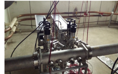
Fermilab SEY measurement stand at MI
