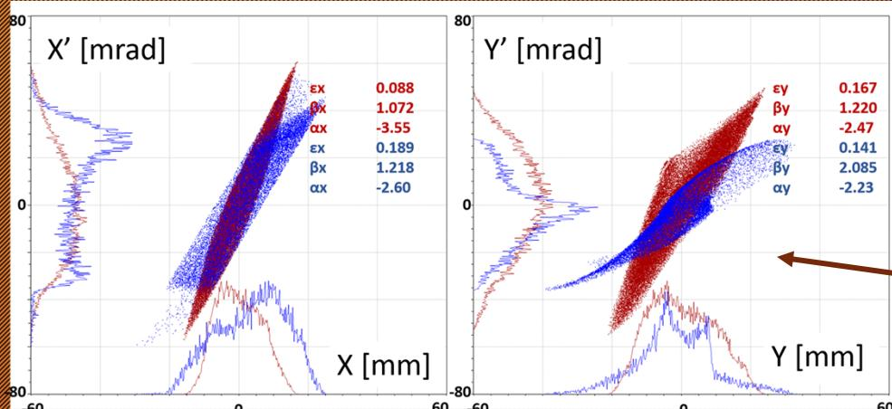
Mismatch between beam phase space tomographic reconstruction (red dots) and simulation results, tracking the IBSimu extracted beam (blue dots). Beam at the exit of the spectrometer bend.
