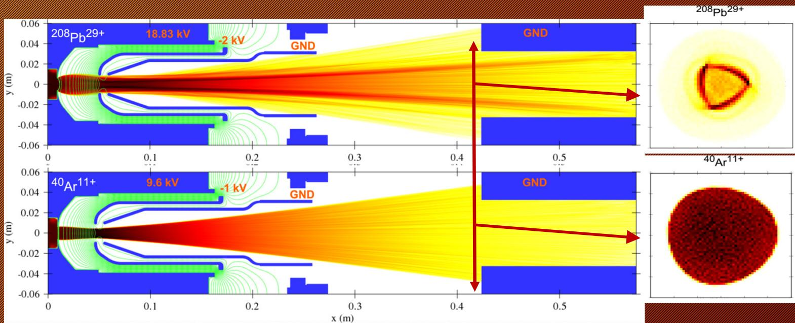
IBSimu ion optical code, 3D magnetic field maps and electrode geometry, full space charge
