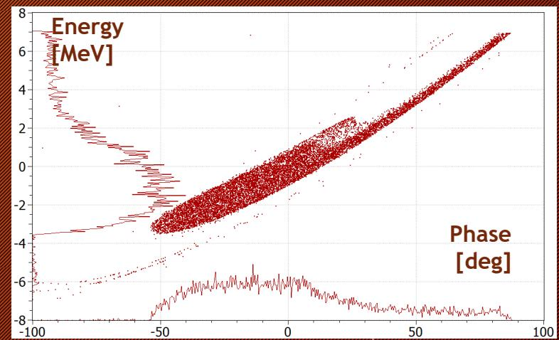
A solution was found on paper to increase the transmission by 20% with new rods design fitting in the same footprint (and slightly lower output longitudinal emittance)
