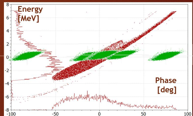
RFQ output longitudinal emittance is tightly contained in the IH acceptance
