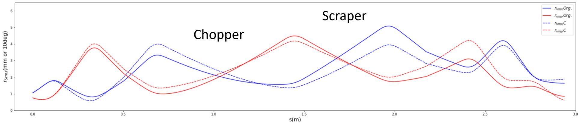
Initial Twiss #2 (improved with new RFQ simulation verified by transverse/longitudinal measurement)
