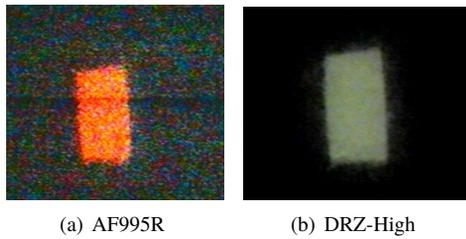
Figure 6: Beam profile obtained with fiber imaging system for (a) AF995R and (b) DRZ-High. Beam shape was uniformed by nonlinear focus.
