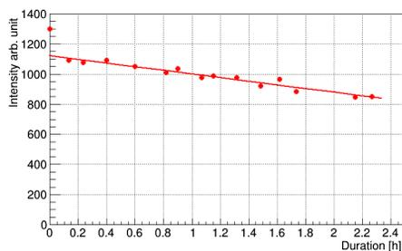
Figure 8: Trend of peak intensity for long duration irradiation of the Ar beam with 75 nA. Line shows result by linear fitting.
