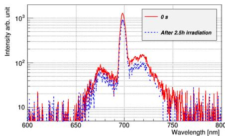
Figure 7: Spectrum of luminescence before and after irradiation of the Ar beam for 2.4 h.
