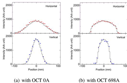
Figure 4: Beam profile obtained with calculations (line) compared with result by the MWPM (dots) supplying current of (a) 0 A and (b) 698 A to octupole magnet. Upper and bottom figure represents for horizontal and vertical directions, respectively.
