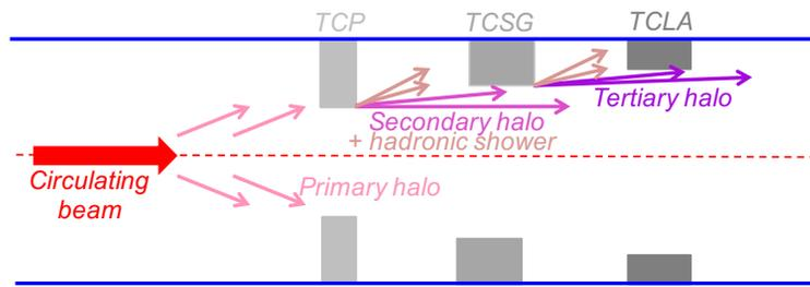
Figure 1: Working principle of the present collimation system.
