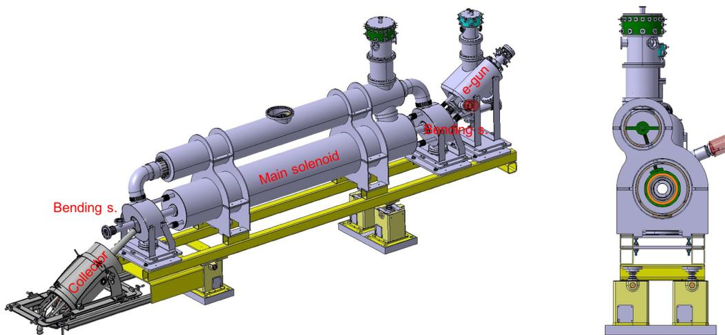
Figure 6: (left) Side and (right) front view of the present HL-LHC hollow electron lens design.
