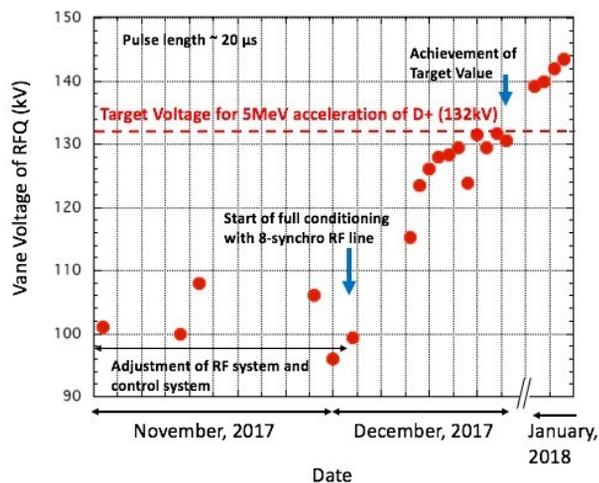
Figure 6: History of RF conditioning id RFQ up to target voltage for D+ acceleration.
