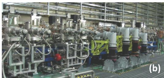
Figure 3: Progress of RFQ installation from (a) April 2016 to (b) June 2017.
