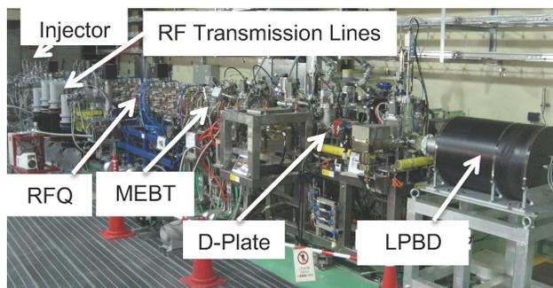
Figure 2: Accelerator components of IFMIF prototype accelerator.
