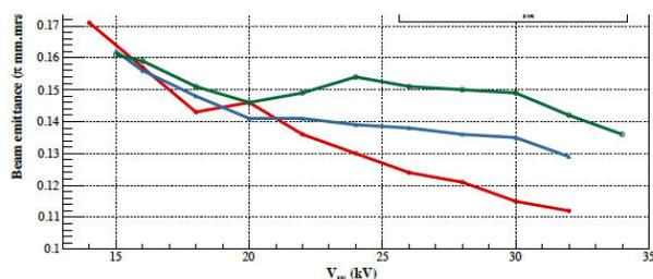
Figure 5: An example of injector beam performance: beam emittance vs. voltage of first extraction gap for D+ beam with energy 100 keV and various extracted beam current, 155, 165 and 175 mA (pulsed beam with 5% duty cycle and 2msec width).
