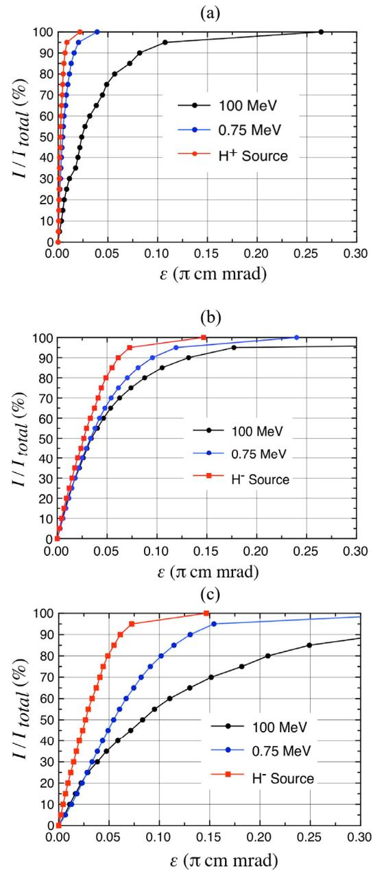
Figure 5: The distribution of the current in the phase space of the different beams in sources, LEBT (0.75 MeV) and after DTL (100 MeV): (a) H<sup>+</sup> beam, (b) H<sup>-</sup> Lujan/pRad/UCN beam, (c) H<sup>-</sup> WNR beam.
