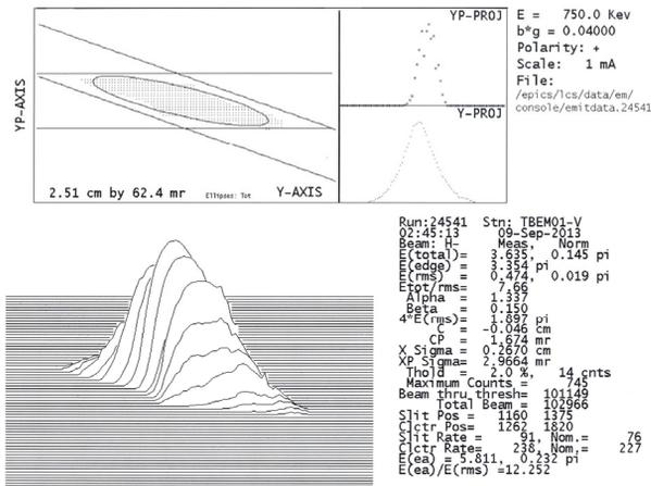
Figure 4: Emittance measurement of H<sup>-</sup> beam at the beginning of Low Energy Beam Transport.
