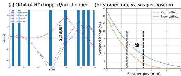
Figure 12: A trial optimization for horizontal envelop at scraper.
