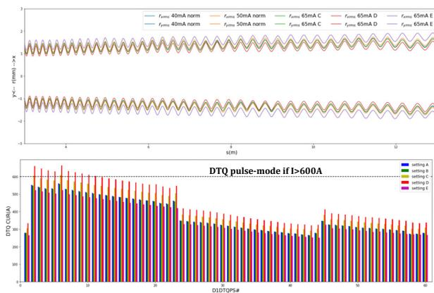
Figure 3: DTL lattice preparation, beam envelope (5\*rms) and operational DTQ current.
