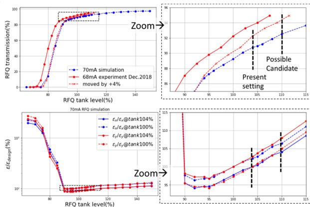
Figure 9: A more realistic RFQ simulation compared with measured transmission.
