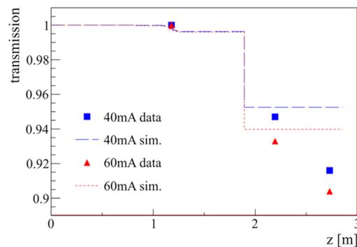
Figure 10: RFQ transmission measurement and simulation.
