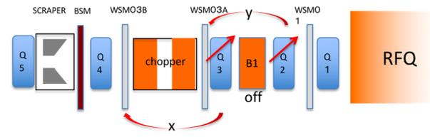
Figure 4: MEBT1 Q scan scheme for transverse measurement.
