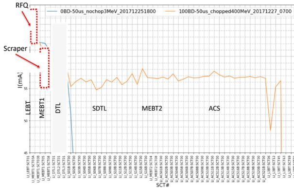
Figure 7: Transmission measured 60 mA trial in December 2018.
