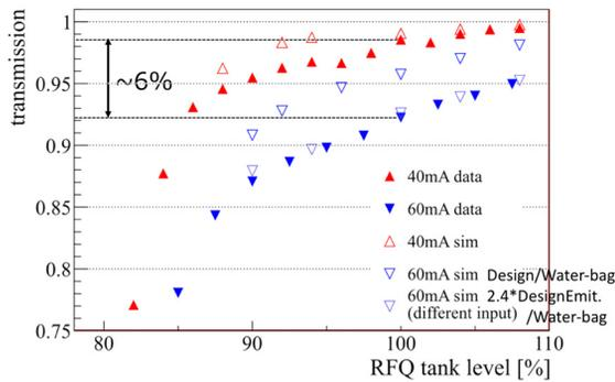
Figure 8: RFQ transmission measurement and simulation.
