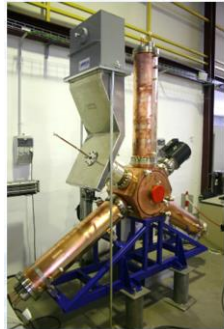
the EU-HOM damped cavity (F. Marhauser et al., EPAC2000, E. Weihrer, TUP5A01 and EPAC08, THXM03)
